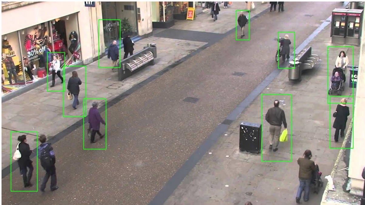
Figure 26: Pedestrian detection with SVM using HOG features [51]
