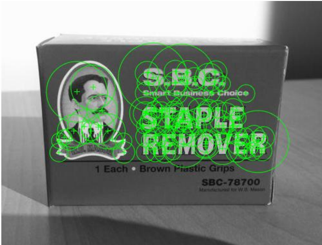
Figure 27: Extracting the most notable features in the box image [52]
