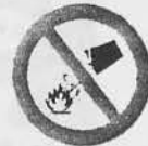
EP 1 P/4 Do not use water to extinguish
