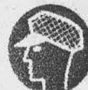
EP 1 M/18 Harnesses/hoods must be worn
