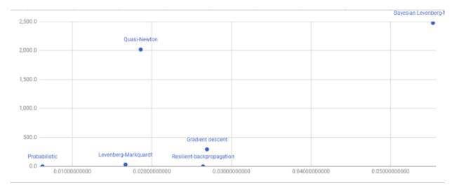
The X axis represents the mean squared error rates, while the Y axis the training time in seconds. The ideal network would appear on the (0,0) position, and as one may see the probabilistic neural network is the closest to the ideal one. The exact performances are as follows:
