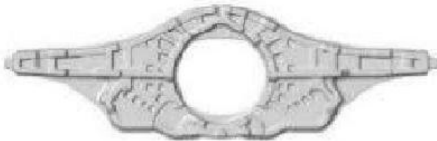
STOVL 472 bulkhead, 19.5 x 6.5 x ft
