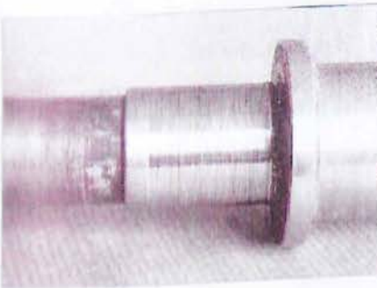
(e) Axle of a hot water circulator (rubbing on a graphite bearing); abrasion by oxide particles embedded in the bearing
