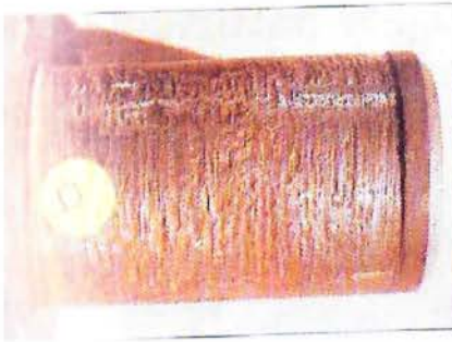
(a) Shaft of nitrided steel; bearing of steel 100 Cr6. Environment: water filled with sand. V = 20 \text{ mm s}^{-1} , P = 20 \text{ MPa}
