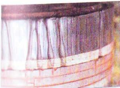
(c) 'Sloodge' pump piston; erosion by the fluid filled with alumina
