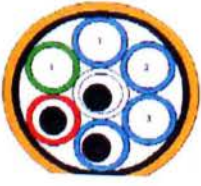
Sub divided Sub-duct
