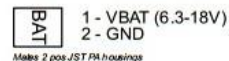
Mates 2 pos JST PA housings Part # PAA-02V-S(P) Crimp terminals Part # SP149-001T-P0.5 (for AWG 22-26 wire)
