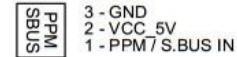
Mates 3 pos servo cable. Solder cables into the holes and connect RC receiver with it. Fits 0.1" header (both straight and right-angle)
