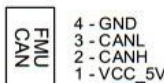
Mates 4 pos Hirose DF13 housings Part # DF13-4S-1.25C Crimp terminals Part # DF13-2630SCF (for AWG 26-30 wire)
