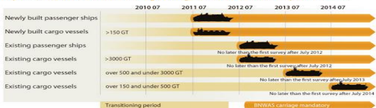
Implementation schedule of Bridge Navigational Watch Alarm System (BNWAS)
