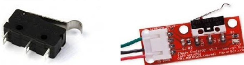
Εικόνα 14 – Mechanical endstop and pcb board with led indication
