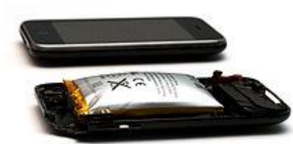
IMAGE 5.3: Apple iPhone 3GS's Lithium-ion polymer battery, which has expanded due to a short circuit failure.
