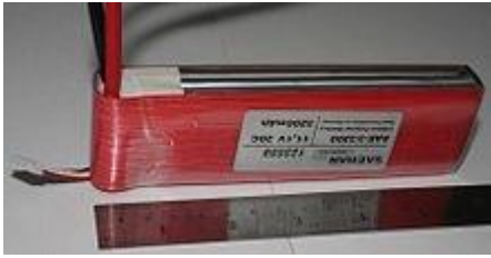
IMAGE 5.2: LiPo battery for RC-models
