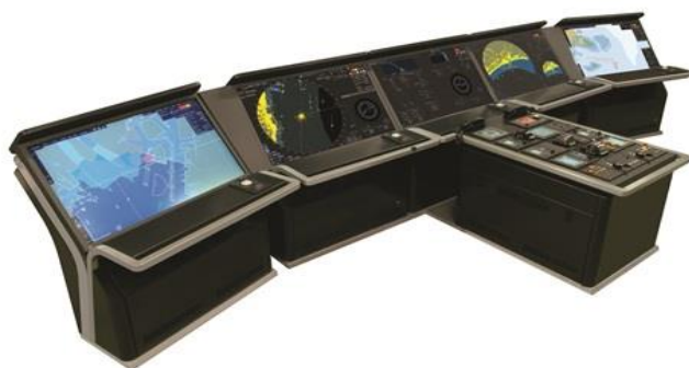
Figure 1: Typical layout of a merchant ship's Integrated Bridge System
