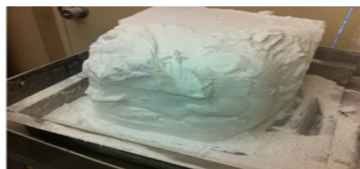
Excess un-sintered powder is removed from parts surface
