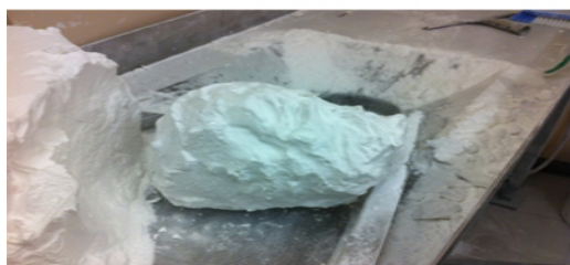
Part is sand blasted to remove the all un-sintered Nylon.
