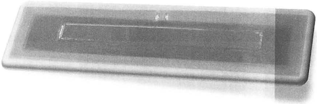
Figure 95: The difference between the external and internal layers of Kapton is more visible with the first manufacturing attempts. The interaction point of the external layers is what holds the assembly together.
