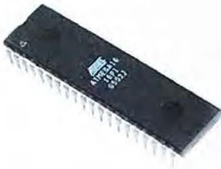
1.3.1 Atmel AVR ATmega16 in 40 pin DIP
