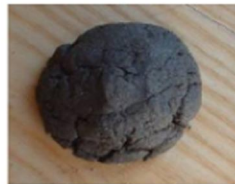
4-15: This drop test soil may have too much clay
