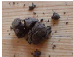
4-14: This drop test is good soil for earthbag
